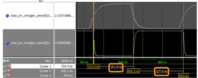
Figure 9 Waveform of RNM Simulation
