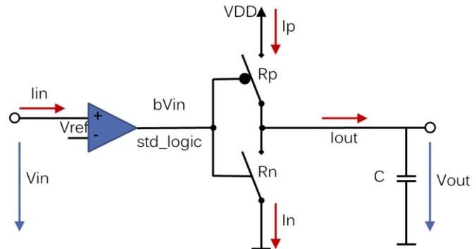
Figure 3 RNM & Switch Level Modeling
